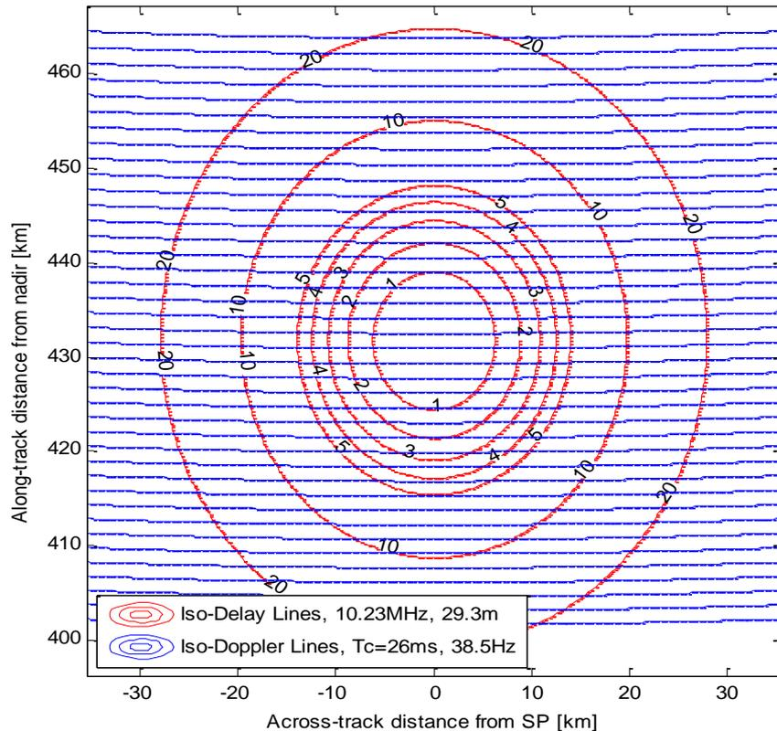
GPS-Galileo L5-E5a Doppler Waveforms, 39 Doppler Bins,  $T_c=26\text{ms}$ , 38.5Hz
