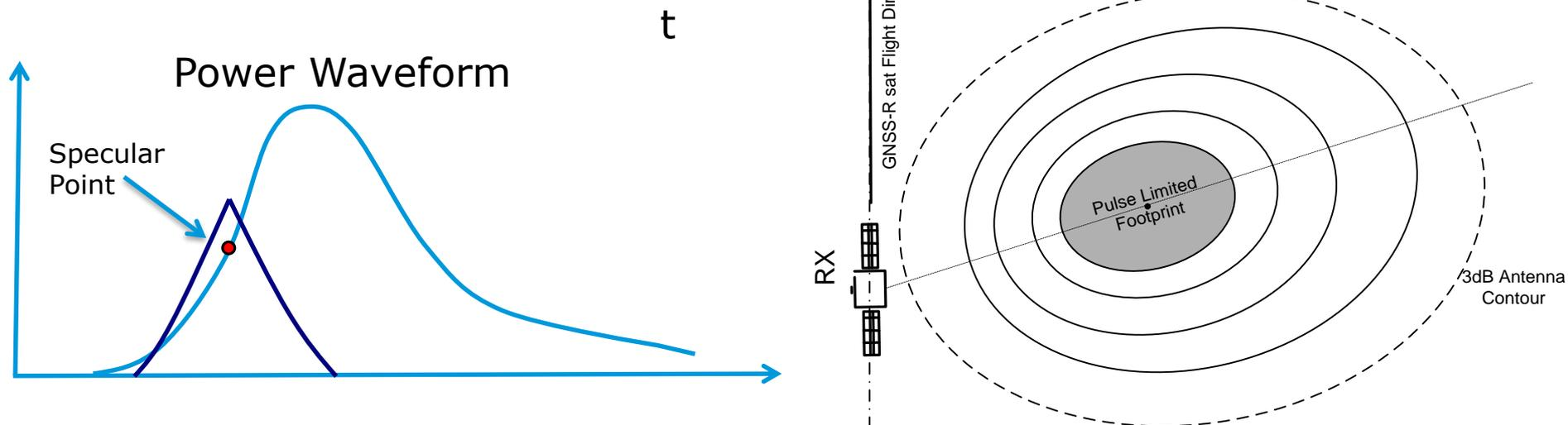
1. The proposed delay-Doppler processing performs **N parallel cross-correlations** at different Doppler frequencies, thus generating a Delay-Doppler Map. The number N is chosen to observe an ocean region as large as the antenna pattern of the GNSS-R receiver, which is much larger than the pulse limited footprint.
