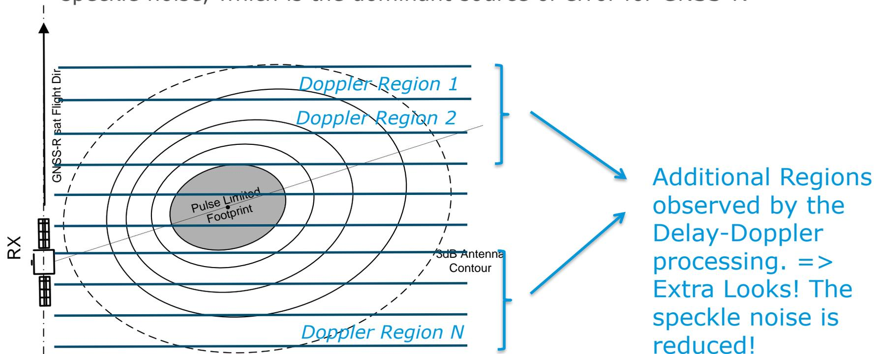
1. The proposed delay-Doppler processing performs **N parallel cross-correlations** at different Doppler frequencies, thus generating a Delay-Doppler Map. The number N is chosen to observe an ocean region as large as the antenna pattern of the GNSS-R receiver, which is much larger than the pulse limited footprint.
