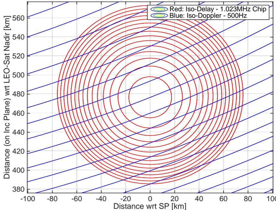
GPS-Galileo L5-E5a Doppler Waveforms, 39 Doppler Bins,  $T_c=26\text{ms}$ , 38.5Hz
