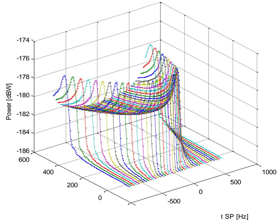
$$DM(\tau) = \langle Y(\tau) \rangle = \iint_{\theta, \varphi} P_r(\theta, \varphi) |U(\tau - t_r(\theta, \varphi), f_d(\theta, \varphi))|^2 d\Omega,$$
